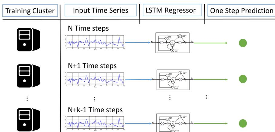
Figure 1: Parallel Training Each RNN Regressor in the HPC Cluster.
